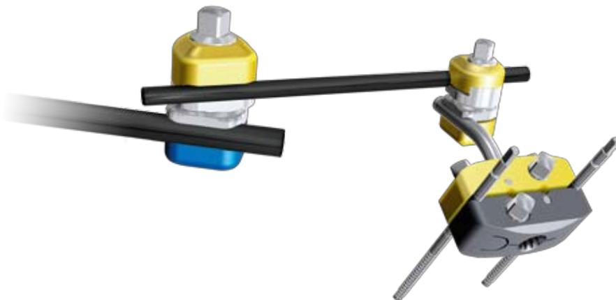
The Hoffmann II Compact  $\varnothing 5\text{mm}/\varnothing 8\text{mm}$  Rod to Rod Coupling can be used to connect the Hoffmann II Compact 5mm Rods to a Hoffmann II  $\varnothing 8\text{mm}$  Rod. This can be helpful in a Foot/Ankle Frame or to connect a humerus frame to a radius frame. The coupling is tightened with a 7mm Wrench.
